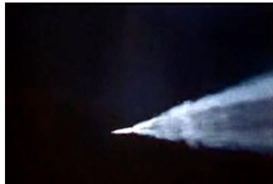
Image 1b. Rocket flight four frames after cutting off the first stage engines. Second stage ullage-rockets have been ignited.
