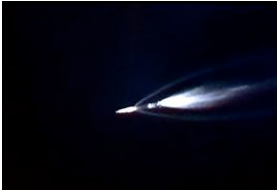
Image 3c. The gap grows larger. The second stage engines exhaust plume is visible in the gap between the stages.
