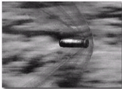
Image 5. A projectile flying at supersonic speed. The trailing "whiskers" are air shocks acquiring a cone shape at a certain distance from the body. A normal shock wave is visible at the front of the blunt head.
