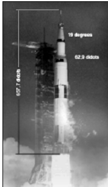
Image 6. Measurement of Apollo to Saturn V booster adapter angle. The linear dimensions measured in pixels are presented in the photo: the rocket height with its needle (110m) and the second stage tank diameter (10.1m). A good (within 5%) match of the vertical and horizontal dimensions ratio shows that the angle of the cone adapter is not distorted in this photograph.
