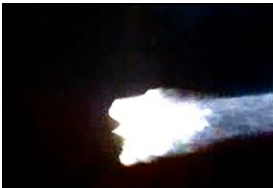
Image 2c. Shock front and the cloud of solid propellant products are catching up with rocket head (frame 192).
