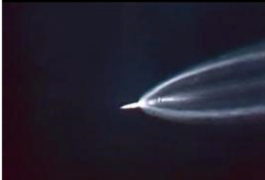
Image 3a. A bright glow is observed in the gap between the stages, indicating that the second stage engines have ignited (frame 266).
