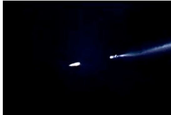
Image 3d. The distance between the stages is now significant. The first stage plume brightness abruptly diminishes – this is 13 secs after the retro-rockets have fired.
