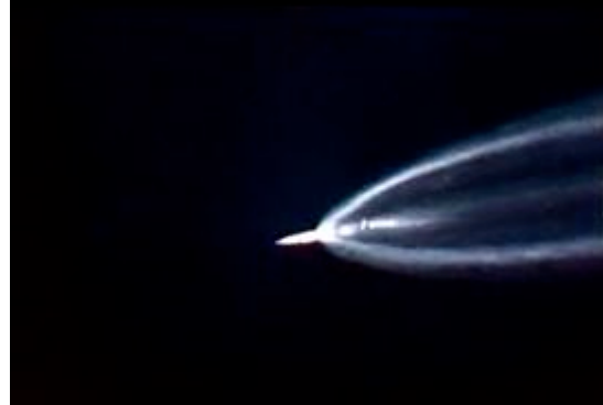
Image 3b. The gap between the stages is increasing. The compression shock begins to lose brightness.
